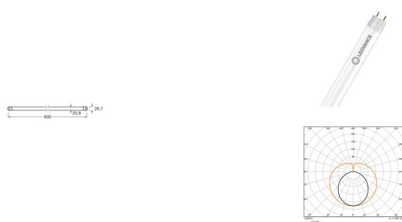
**Scheda tecnica Ledvance Tubo LED T8 EM Performance Conventional (EM), Mains (AC) High Output T8 7W 1100lm - 840 Bianco Freddo | 60cm - Sostitutiva 18W**
