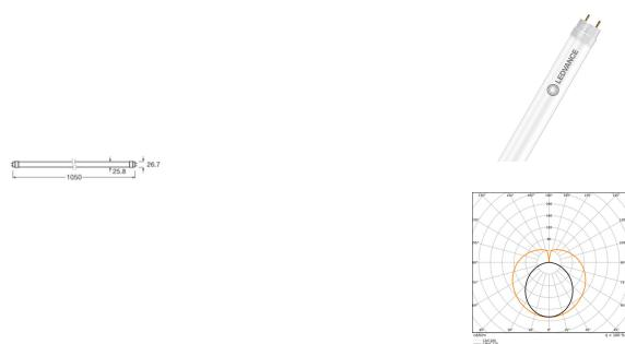
**Scheda tecnica Ledvance Tubo LED T8 EM Superior Conventional (EM), Mains (AC) High Output T8 11.4W 1800lm - 830 Luce Calda - | 105cm - Sostitutiva 38W**
