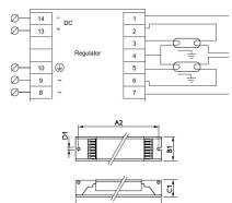
Scheda tecnica Philips HF-R 258 TL-D EII 220-240V for 2x58W
